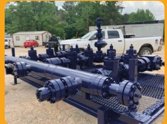
Figure 1: Well Control manifold
